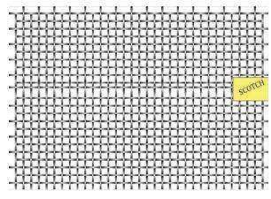
If the mesh is supplied in a roll, the imperfections will be marked on the edge of the mesh with adhesive tape.
