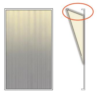
LED light perpendicular to woven metal mesh
