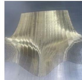
Warp is more flexible than weft (more malleable), although it is still at risk for deformation (shape memory)
