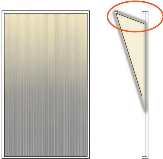
*LED light perpendicular to woven metal mesh*
