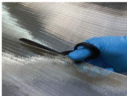
Place guides with paper tape to hold the wire before cutting along the weft (preferred method for cutting against the warp strands)
