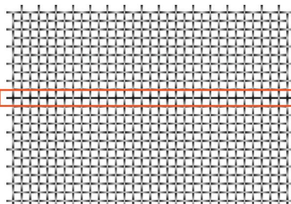
This is the natural feature of the metal mesh, which stems from the hoven process. It could be recognized as an imperfection if this feature is replicated every 3.3 meters (~10.8 ft) on the wide of the mesh.
