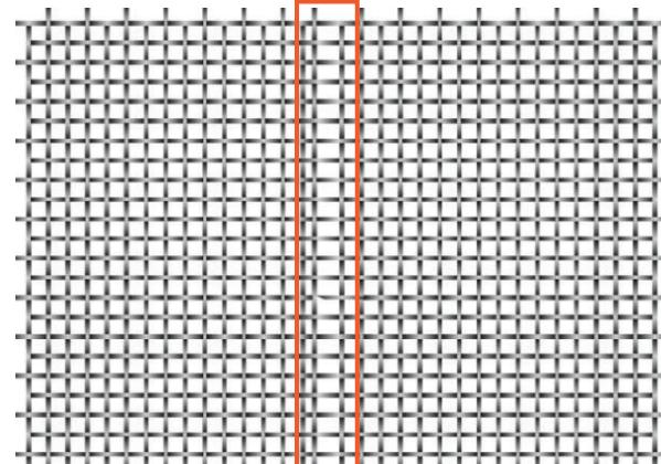
These gaps can occur on the warp and weft of the mesh and its caused by the wire breaking during the weaving process. These could be recognized as imperfections if these features are replicated every 3.3 meters (~10.8 ft) on the wide of the mesh and/or every 30 cm (~11.8 in) on the length of the mesh.
