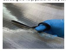
Place guides with paper tape to hold the wire before cutting along the weft (preferred method for cutting against the warp strands)
