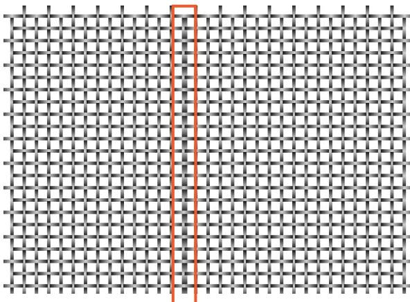
The metal mesh can have a section with warp roughness. It could be recognized as an imperfection if this feature is replicated every 3.3 meters (~10.8 ft) and its more than 30 cm (~11.8 in) on the length of the mesh.
