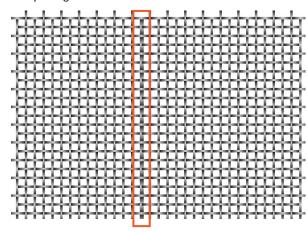
The metal mesh can have a section with warp roughness. It could be recognized as an imperfection if this feature is replicated every 3.3 meters ( $\sim$ 10.8 ft) and its more than 30 cm ( $\sim$ 11.8 in) on the length of the mesh.
