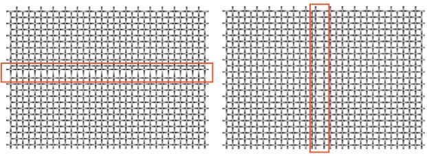
These gaps can occur on the warp and weft of the mesh and its caused by the wire breaking during the weaving process. These could be recognized as imperfections if these features is replicated every 3.3 meters (~10.8 ft) on the wide of the mesh and/or every 30 cm (~11.8 in) on the length of the mesh.
