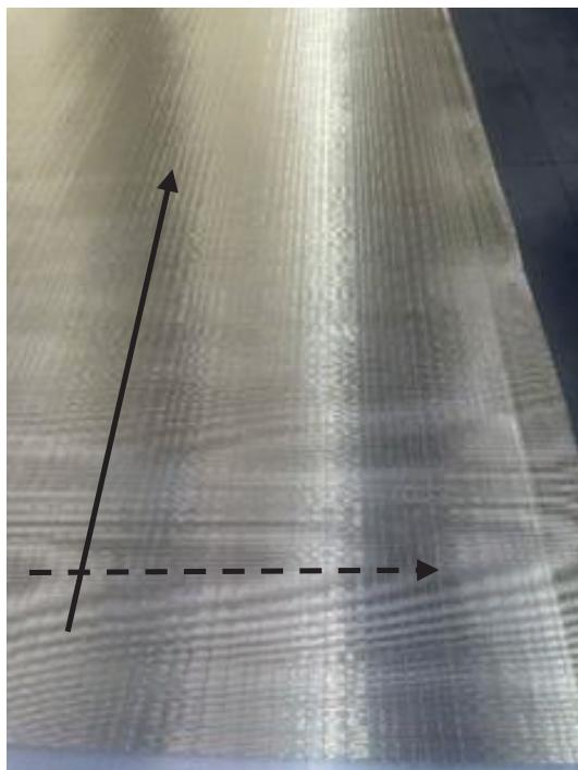
Weft is rigid, so the mesh can be deformed due to its metallic nature (mind the shape memory)
