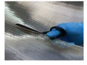
To cut along the weft is preferred to place guides with paper tape to hold the wire.
